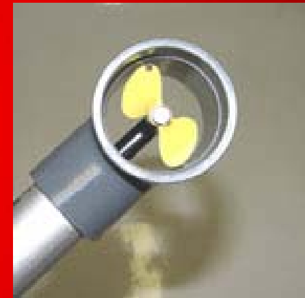
Flow Probe measures water velocity
