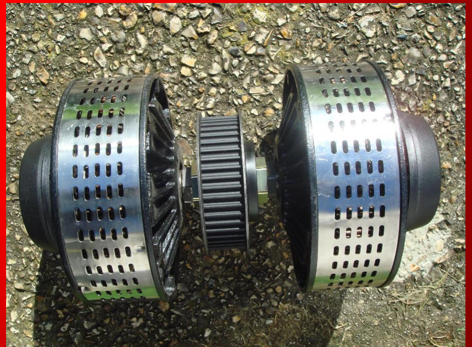
Two Agni 143 motors in one pulley Courtesy of Cedric Lynch
