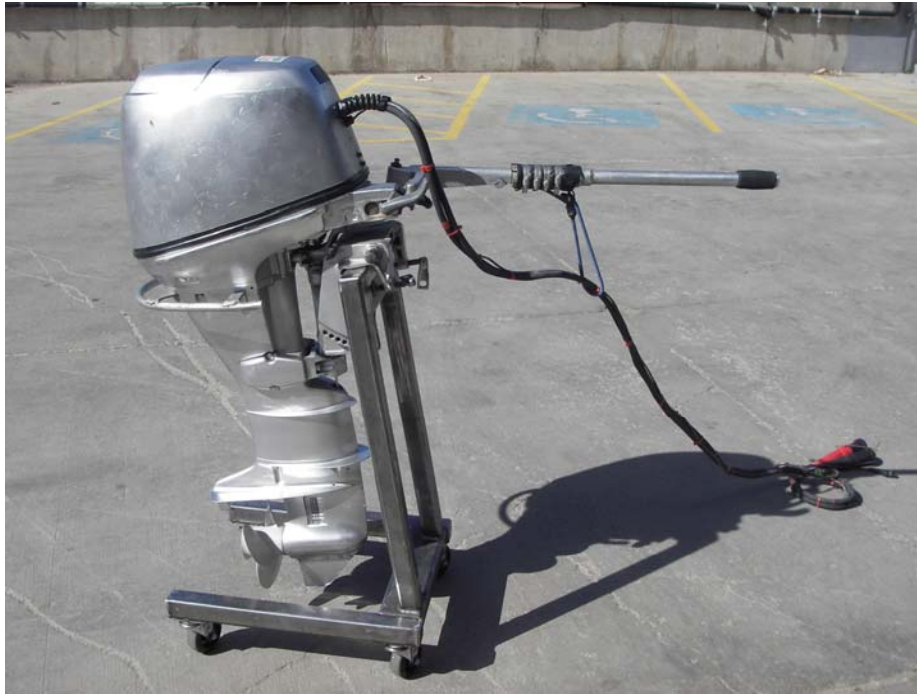
Figure 3 - Motor System Enclosed in Cowling
