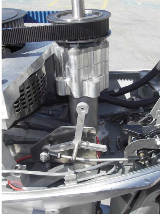
Figure 5 - Throttle Linkage to Actuate Motor Controller Potentiometer
