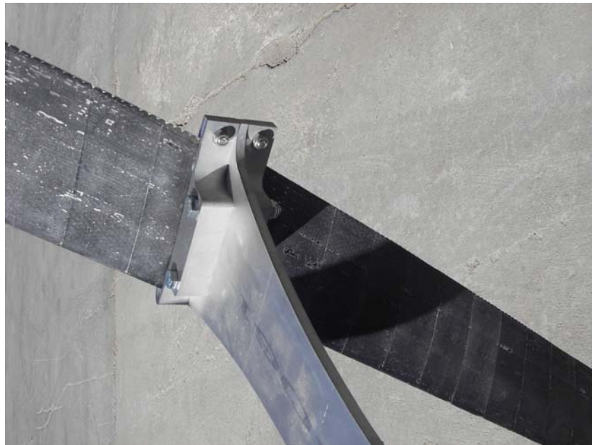
Figure 7 - Helical Blade Section Coupling
