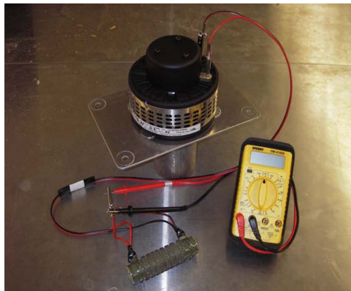
Figure 14 - 3.1 ohm Power resistor circuit
