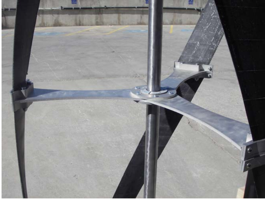
Figure 8 - Blade Hubs and Support Arms
