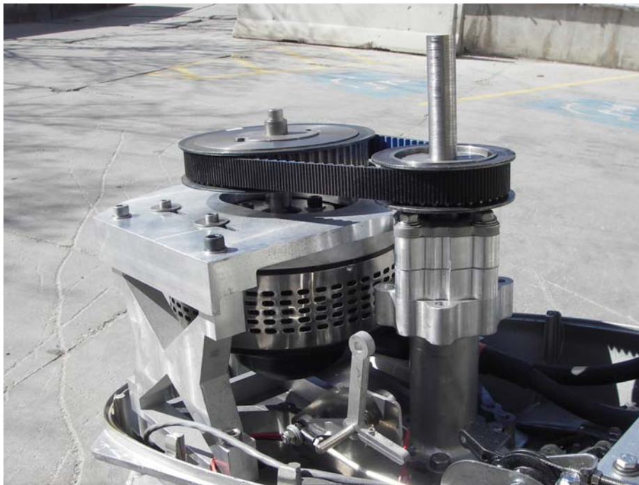
Figure 4 - Motor with Bearing Carrier and Adapter Plates
