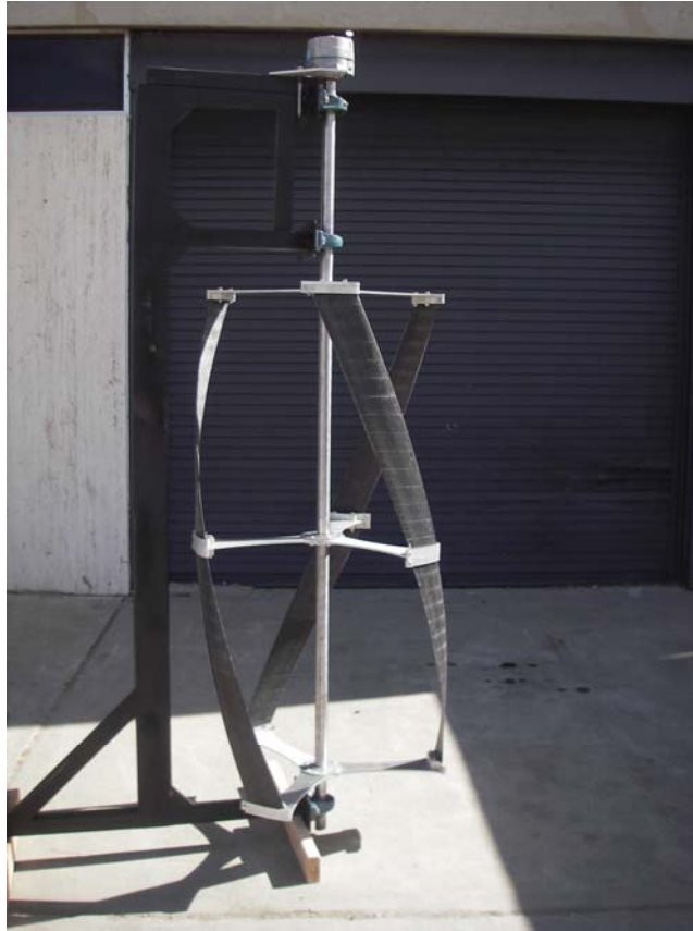
Figure 6 - Gorlov Turbine Assembly with Generator
