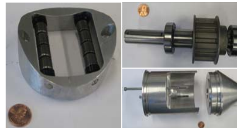
Figure 2: lower belt-guide journal (left); input shaft (top right); propeller shaft housing assembly (bottom right)
