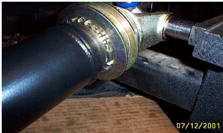
Figure 9.3 Coupling and shift collar assembly welded to the drive shaft
