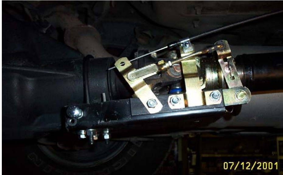
Figure 9.5 Shift linkage, collar and coupling apparatus
