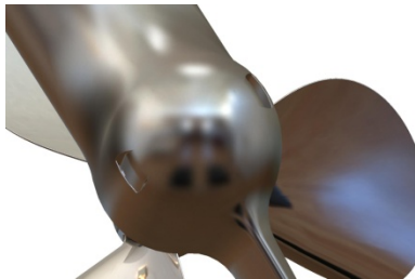
Figure (15) Water Intake Slots for Cooling
