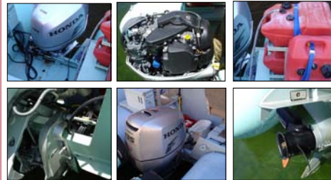
Figure 1. Hydraulic Steering, Current Engine Configuration, Fuel Storage, Lower Unit Mount, Engine Compartment Configuration, Composite Propeller
